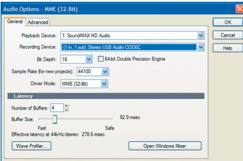
For Playback Device, select your soundcard. For Recording Device, select: Stereo USB Audio CODEC.- After selecting this output you may monitor the recording via the RCA output on the T.92 USB.
