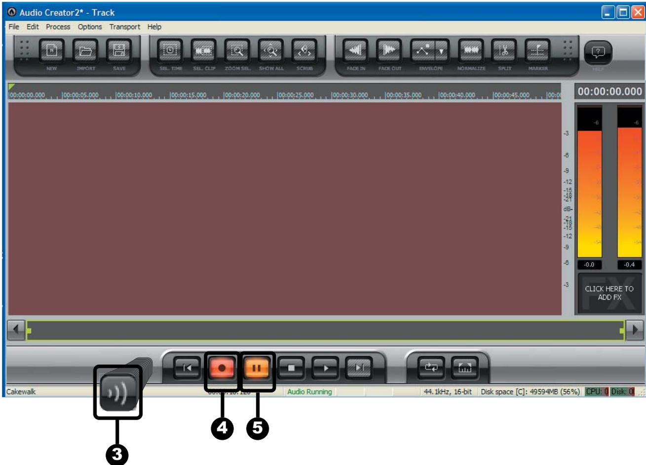
3. Press the (3) Input Monitoring button. This will allow you to listen to the audio as you record it from the T.92 USB.
