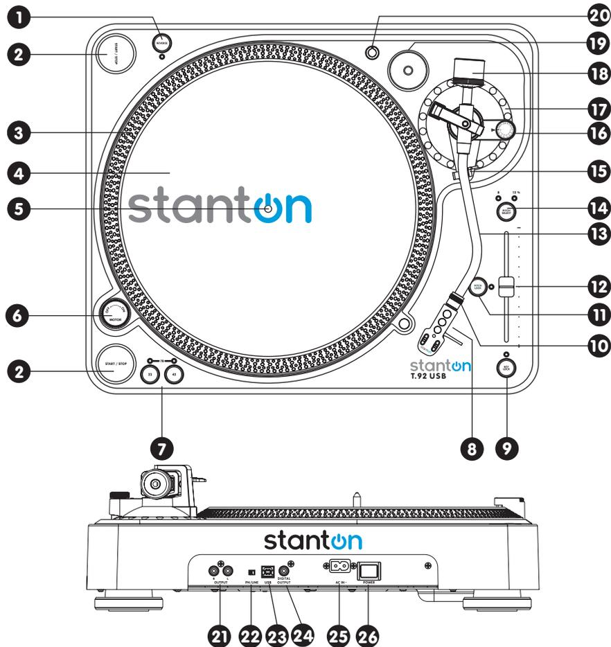
1. **REVERSE** - This button is used to reverse the direction of the platter rotation.
